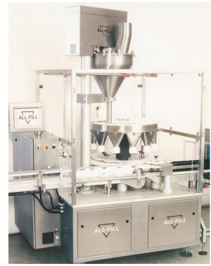
12 pocket continuous motion rotary filler for filling over 500 spice/herb combinations into PET catering jars at 120 jars per minute. Features the All-Fill "fully sealed" filling system, adjustable vibration settling, checkweigher feedback and touch-screen control.
