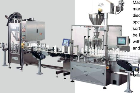
Machines are selected from specialist manufacturers following detailed discussions with the client to establish a specification. Functions such as container sorting/cleaning, capping and labelling can be incorporated into the filling line together with powder bulk feeding, metal detection and check-weighing systems.
